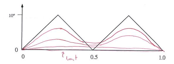
b. A one meter metal rod initially has the temperature distribution shown below. Suppose the ends are insulated. As  $t\to\infty$  what will the temperature distribution approach? Graph this and sketch graphs for several intermediate temperature distributions we would expect to see.
