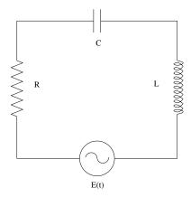
Here R is resistance, L is inductance, C is capacitance, and E(t) is an external applied voltage. Let Q(t) be the current. Then recall that this circuit is governed by
