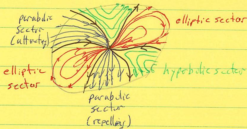
It has six sectors, two elliptic, two hyperbolic, and two parabolic. The solution curves that divide the sectors are called separatrices.
