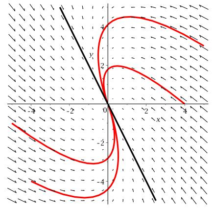
The origin in this case is called an improper node. It is asymptotically stable. It looks like it wants to be a spiral, but could not make up its mind!
